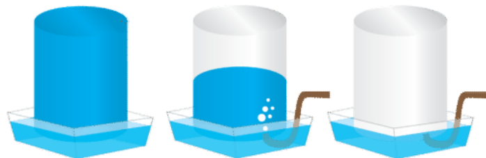
Figure 7.6 A gas produced in a chemical reaction can be collected by water displacement.
